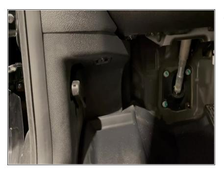
Turn ignition off and plug OBD programmer into OBD port
