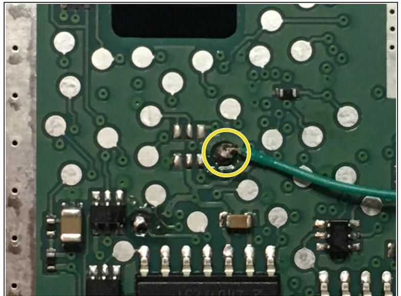
ⓘ The SKSNG205D4 comes with a jumper wire. There are 2 points on the EIS board that the wire needs to be soldered to.
