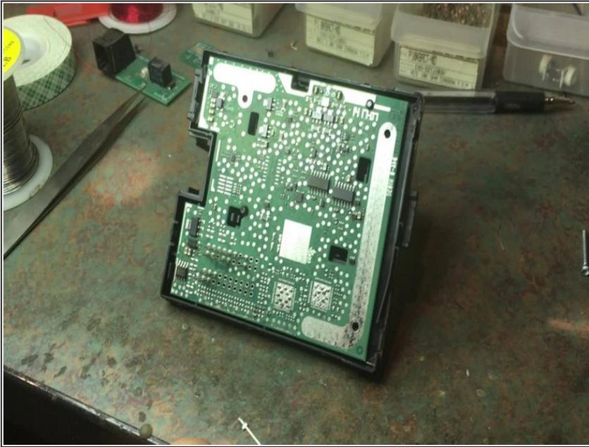
**⚠ The EIS circuit board has static sensitive components. Be sure to use proper grounding practices when working with this board**
