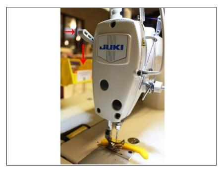
Behind the machine there is a lever that can be pushed up or down. This is to lower the presser foot to allow more space around the needle.
