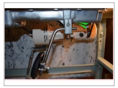
Below the table, there should be a knee lifter on the right. This lever is to create space so that the fabric
