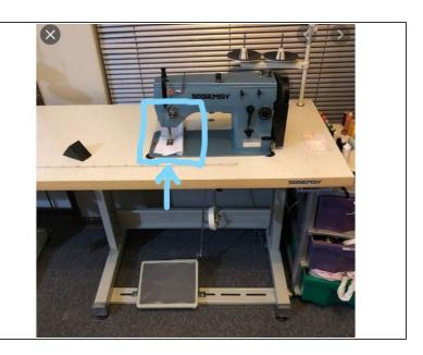
• Press knee on the knee lifter and use the knob on the right side to let space in so that the fabric can be inserted in.
